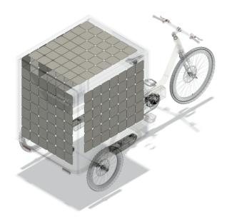
By integrating 550 Wp of solar cells into the cargo box body, your cargo bike can operate for several months without requiring a battery recharge from the grid.
